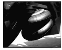
The DUNLOP Type Air Springs can be mounted either individually or in panels (where the requested number of air springs is connected), depending on the vehicle (device) weight. The rubberized-fabric wall of the body must not come into contact with sharp or hot objects (iron scale, edges, exhausts, etc.). The Air Springs can be inflated either individually or centrally. It is recommended to connect them to the source of pressurized air via a control valve.
